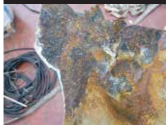
EXTERNAL CRACKS IN EXISTING SYSTEM AND SPREAD OF CORROSION UNDER FILM
